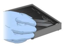
4 Place each BeadChip into a black frame, aligning the barcode with the alignment fixture ridges. Fully submerge each BeadChip.
