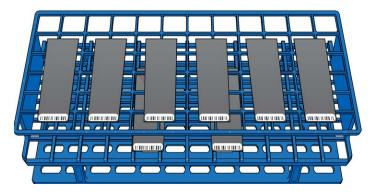
Proper BeadChip placement prevents wicking, uneven drying, and pooled dye protectant.
