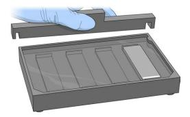
7 Place a clean glass back plate on top of each clear spacer. Position the plate reservoir at the barcode end of the BeadChip, facing inward to create a reservoir against the BeadChip surface.
