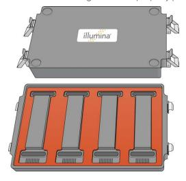
5 Add 400 µl PB2 to the top and bottom wells of each beadchip subchamber in the hybridization chamber.
