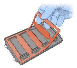
4 Make sure that the gaskets are properly placed and seated.
