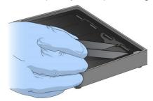
4 Place each BeadChip into a black frame, aligning the barcode with the alignment fixture ridges. Fully submerge each BeadChip.
