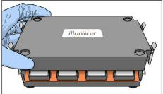
5 Close the hybridization chamber clamps in this order: top-left, bottom-right, top-right, and then bottom-left. Make sure that the lid is secure and even on the base (no gaps).
