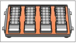
2 Place the back of the lid onto the chamber, and then slowly lower the front to avoid dislodging the inserts.
