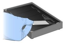
5 Place a *clear* spacer onto the top of each BeadChip. Use the alignment fixture grooves to guide the spacers into position.
