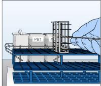
27 Make sure that the staining rack is in the center of the tube rack to ensure uniform coating. Avoid the raised edges.
