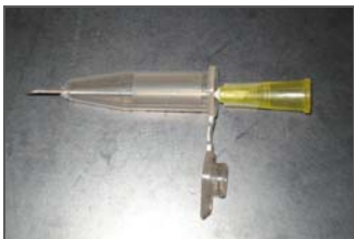
Figure 5 Puncture 0.5 ml Microcentrifuge Tube
