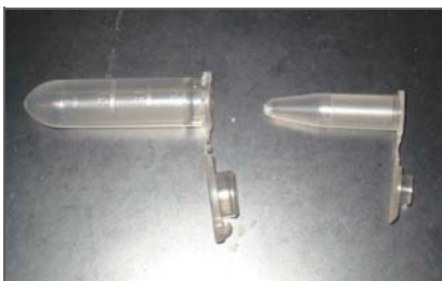
Figure 6 Place 0.5 ml Tube into 2 ml Tube
