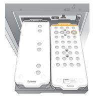
Slide the drawer into the chiller, and then close the reagent chiller door.
