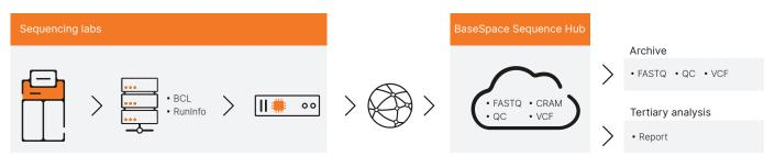
Figure 3: Hybrid cloud DRAGEN secondary analysis deployment — Customers can use a DRAGEN Server to perform primary and secondary analysis, and harness cloud resources, such as BaseSpace Sequence Hub, for multi-sample analysis, data archive, and tertiary analysis.
