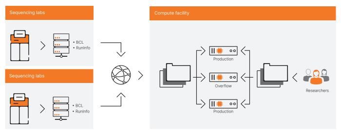
Figure 1: Centralized DRAGEN secondary analysis onsite deployment —Individual labs, each with their own fleet of sequencers, can temporarily store raw sequencer output data on cache storage proximal to their instruments. Data are transferred to a centrally-managed compute and storage infrastructure with DRAGEN Servers. Work queues are managed to maintain production service levels with fail-over capabilities.
